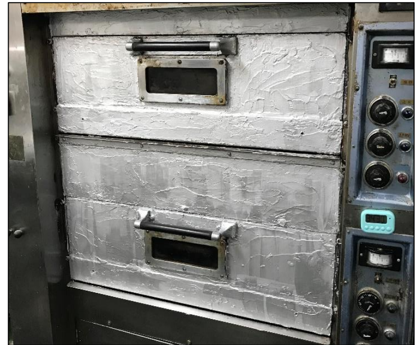
After painting thermal insulation paint on bread baking oven door
