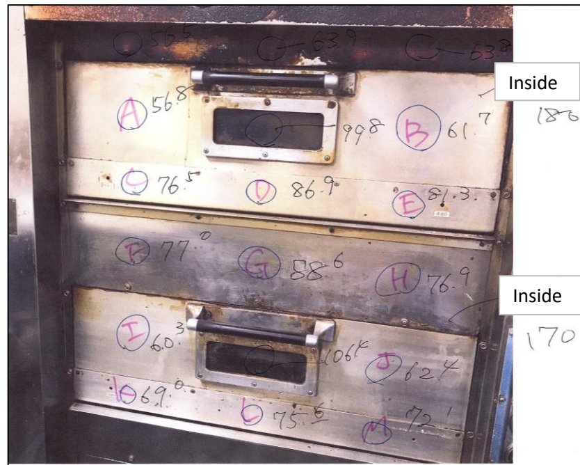
Bread baking oven door(Place for temp measurement )
